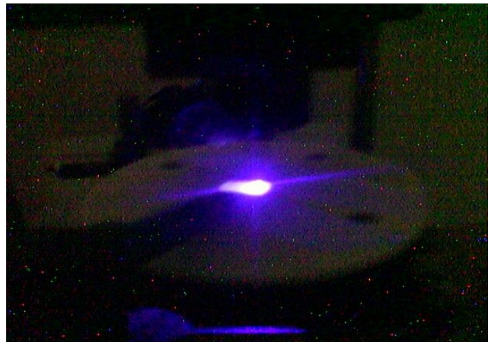
Figure 2: Optically pumped GaN laser, emitting at 408 nm.
